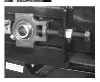
Conveyer Belt Adjustment is easily made by a single adjustment bolt on the left and right sides of the machine. First, loosen the jam nut and begin tightening the adjustment bolts. The belt should have some "play" in it. Each side should be adjusted the same, with the same distance between the bolt head and the front of the adjustment block. Having the adjustment equal on both sides is critical for proper belt tracking and acceptable service life of the belt.
