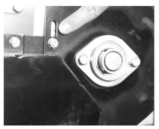
11 Brush Adjustment - The brush can be adjusted by loosening the nuts on the brush slide (one on each side of the unit). Push down on the brush assembly until the brush makes light contact with the conveyor belt,
