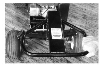
Forward/Reverse - To move the unit forward, push down on the steering handle. To steer the unit, simply move this handle from right to left, depending on the direction in which you wish to travel. To move in reverse, lift up on the handle and steer in the same manner.
