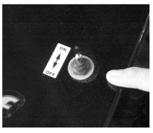
Engine On/Off Switch - After completing all necessary maintenance and making sure the fuel tank is full, start the engine by first positioning the toggle switch in the "on" position.
