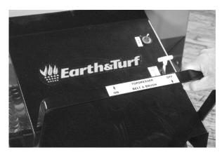
Ready to Spread - When you are ready to spread, you must engage the topdresser engagement lever rearward. To disengage the belt and brush, pull the lever forward. The topdresser will only spread when moving forward. The unit is designed this way so you cannot double-spread when backing into tight areas.
