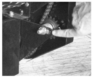
9 Brush Chain Tightness is adjusted by loosening the idler sprocket on the lower right side of the machine (viewed from behind the unit). Push the idler forward to tighten the chain, then re-tighten the idler bolt.
