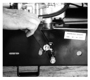
3 Release the Parking Brake by moving the lever backwards to the "off" position.
