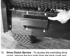
Drive Clutch Service - To access the overriding drive clutch, remove the four bolts from the back cover and remove the cover. This gives access to the clutch should repairs ever be necessary.
