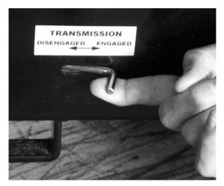
4 Engage the Hydrostatic Transmission by pulling the engagement lever forward. To permit free movement, should it be necessary to push the unit without the engine running, be sure to disengage the transmission by pushing this lever forward.
