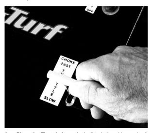
Place the Throttle Lever in the "choke" position and pull the starting rope, which is located just below the throttle control. When the engine starts, move the throttle lever back to the "fast" position.
